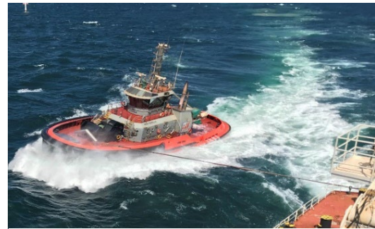
Escort tug in active indirect towing mode Copyright Robert Allan Ltd
